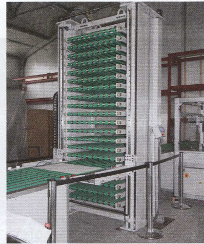
The BMR multi-ream rack is available as a buffer for 10 to 20 reams.
