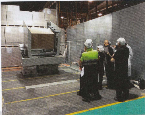
The BSW-AUP pile turner represents the latest generation of the Baumann-Wohlenberg pile turners.
